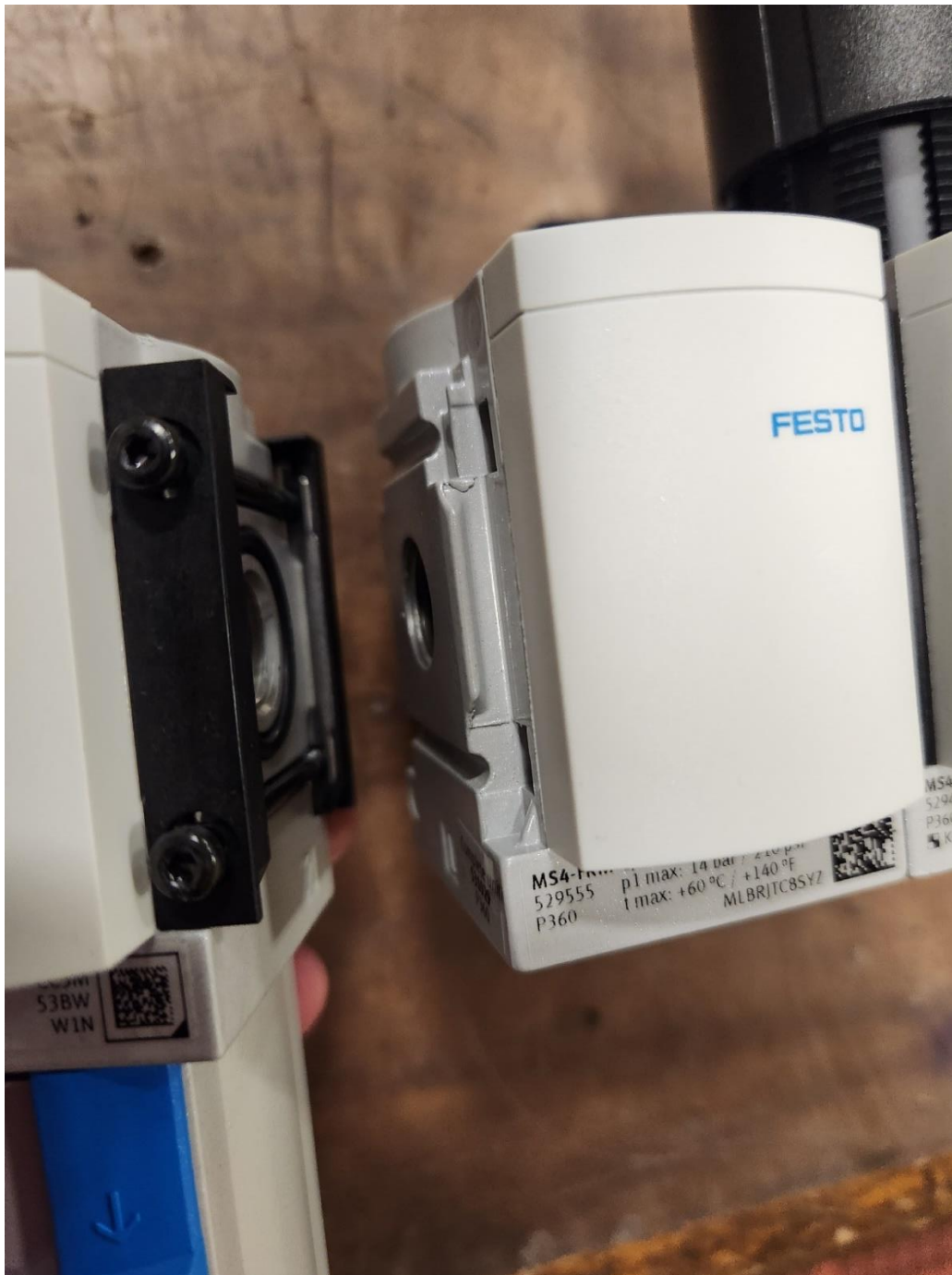
Figure 7: Clamp point of manifold and filter unit
