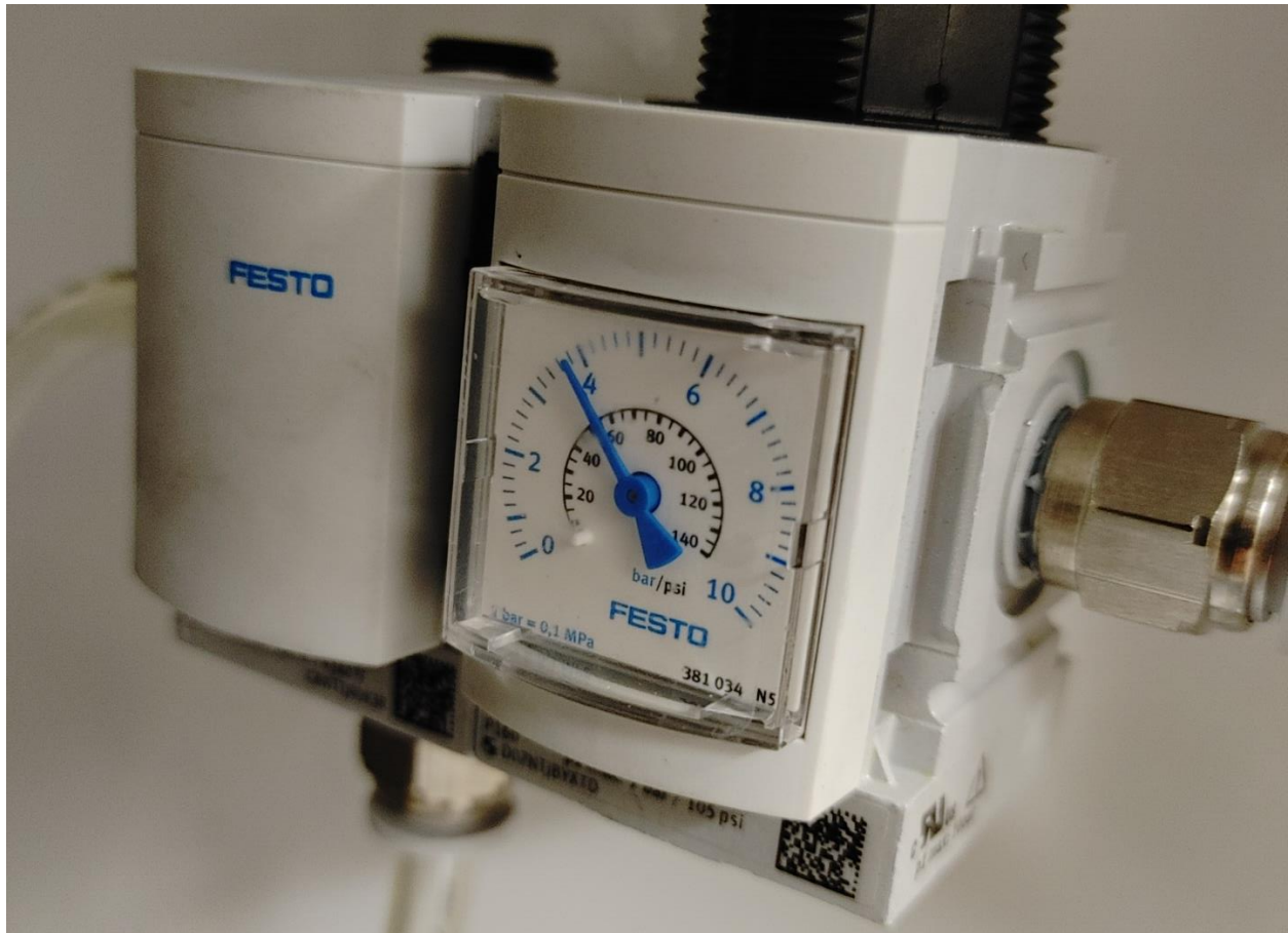
Figure 2: Air prep assembly without filter, manifold on the left, pressure regulator on the right.
